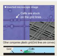
Easier to count because cells do not get stuck on the grid lines that are molded in the groove form. Cells are easier to be
